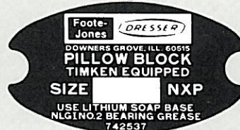
Fig. 7-5: Non-Expansion Type Pillow Blocks are identified by a red name plate like this.
